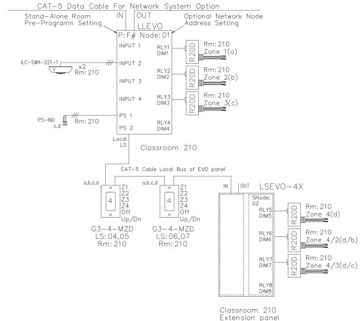
OPERATION: Switch ON/OFF On Level set for 50% dimming Motion sensor set for Vacancy Photo Sensor limits max level in daylight zones
