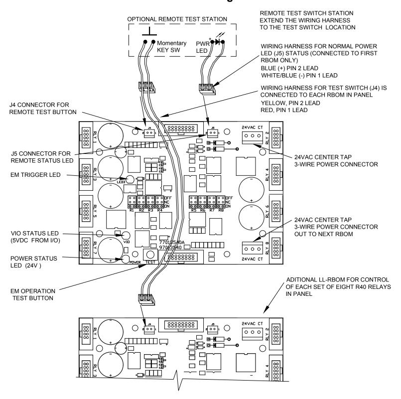
A remote emergency test switch can be connected to the provided wiring harness that comes with the LightLEEDer Emergency UL 924 lighting control panel. The Installing electrical contractor will extend the 22AWG wiring harness leads to the EM test switch location.
